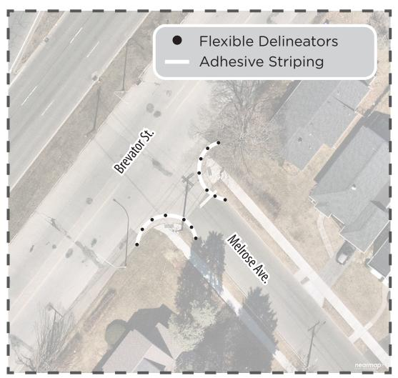
Note 1. Proposed curb extensions will provide at least 20 feet for driving lanes. Note 2. Curb extensions should not extend > 6 feet from the intersection.
